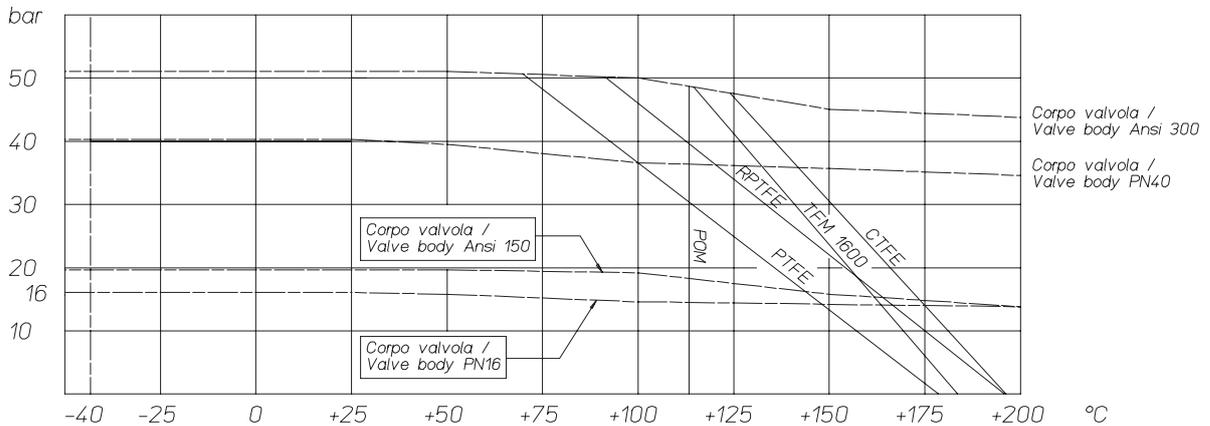
**DIAGRAMMA PRESSIONE TEMPERATURA PER VALVOLE CON CORPO IN ACCIAIO AL CARBONIO TEMPERATURE PRESSURE DIAGRAM FOR CARBON STEEL BODY VALVES**
