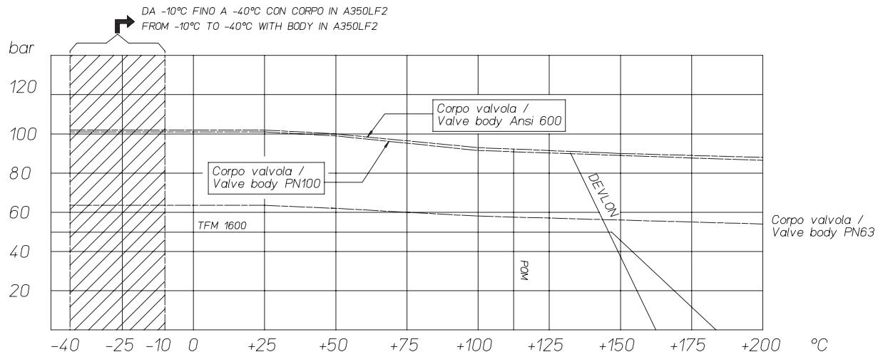
**DIAGRAMMA PRESSIONE TEMPERATURA PER VALVOLE CON CORPO IN ACCIAIO AL CARBONIO TEMPERATURE PRESSURE DIAGRAM FOR CARBON STEEL VALVES**
