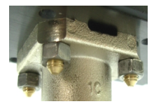
Assembly of pneumatic actuator with M5 nuts
